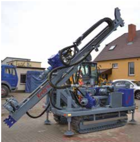
igus® E4 series guides pulsating hydraulic hoses to this pile driver
