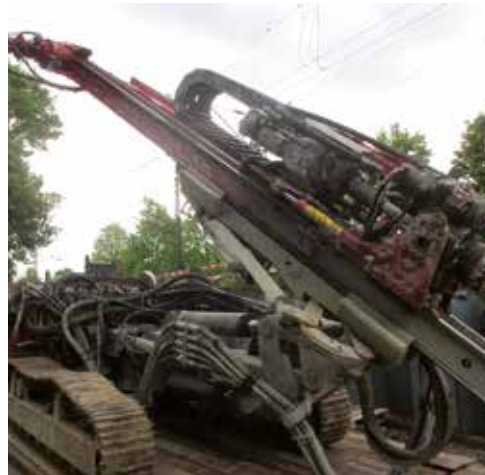
Anchoring drill in operation with igus® E4 e-chain® with dirt and vibration
