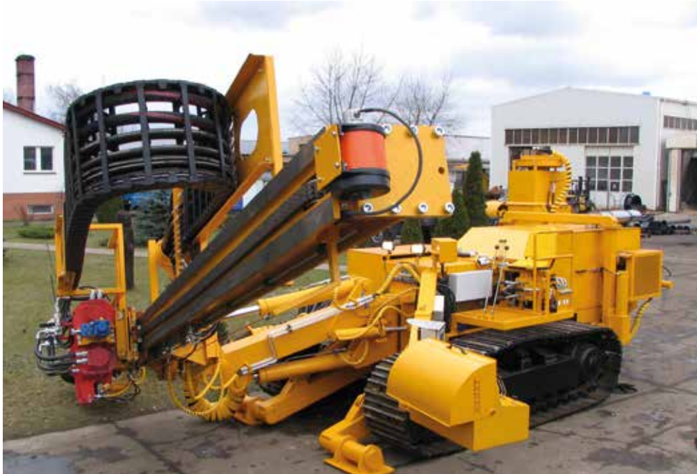
igus® H4 series guides hydraulic hoses reliably in an anchoring drill
