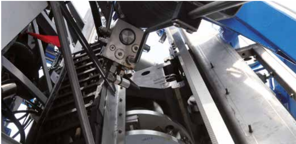
Three E4 series e-chains® supply energy to this drilling equipment working 4,000 m under the sea. Special igus® plain bearings for underwater applications ensure a lubrication-free operation in seawater
