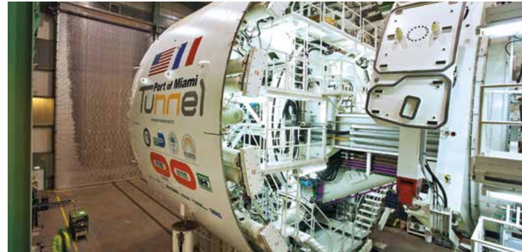
The erector is supplied with energy by two counter-running e-chains®.
