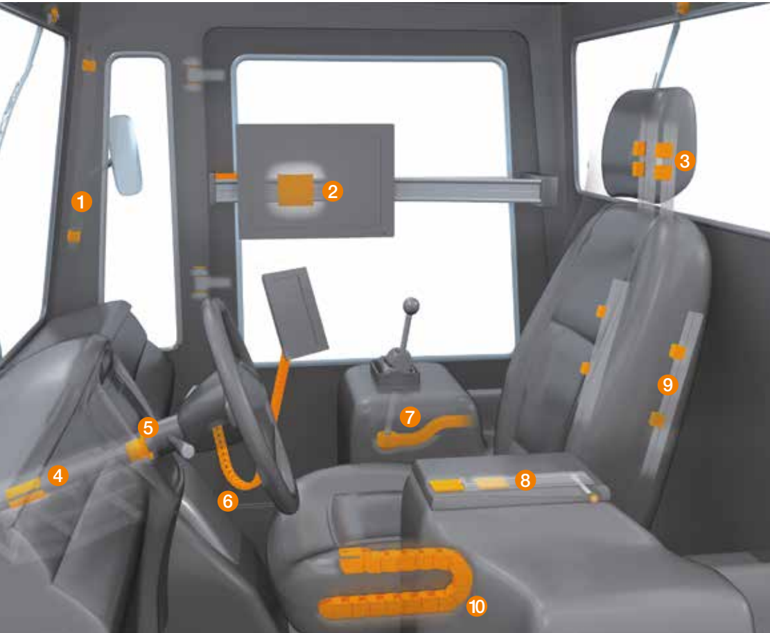
3 Head rest back adjustment drylin® W profile guide
