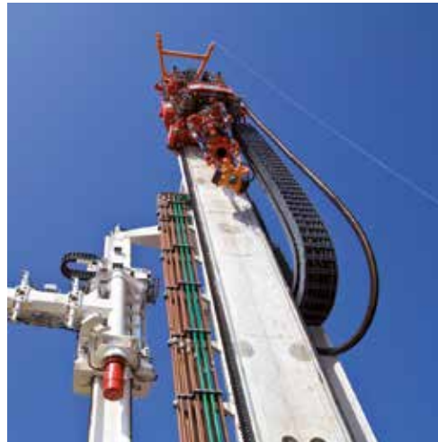
Exploration project in southern Argentina, under extremely challenging conditions, the company has now equipped two drilling systems with custom modified igus® Atex e-chains®.
