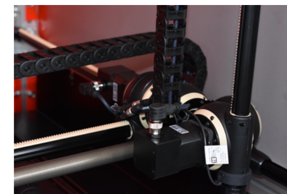
Apero linear robot in the dispensing mechanism of an ice cream vending machine
