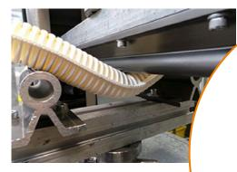
Bending test on the e-skin® soft corrugated tube
