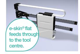
Specialising in the manufacture and development of components for automation technology and a leader in the field of rotary indexing tables, Weiss GmbH needed to find a cable feed-through to the tool centre that could hold two sensor cables and two hoses, each with a diameter of 4mm. The solution was the igus® e-skin® flat cable guidance system. Its service life is over 57 million double strokes
