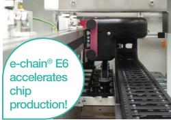
An igus® e-chain® from the E6 range accelerates work processes in the wafer-handling application in chip production. The E6 easily supplies energy for wafer handling in chip production requiring acceleration rates of up to 4m/s² and speeds of up to 6m/s. Its low abrasion is especially important because a high degree of purity is critical in chip production. The E6 is cleanroom-compatible and has Fraunhofer IPA certification.
