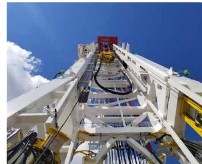
Figure 2: Energy chain system for top drive and pipe handling on a land drilling rig (Source: igus® GmbH)
