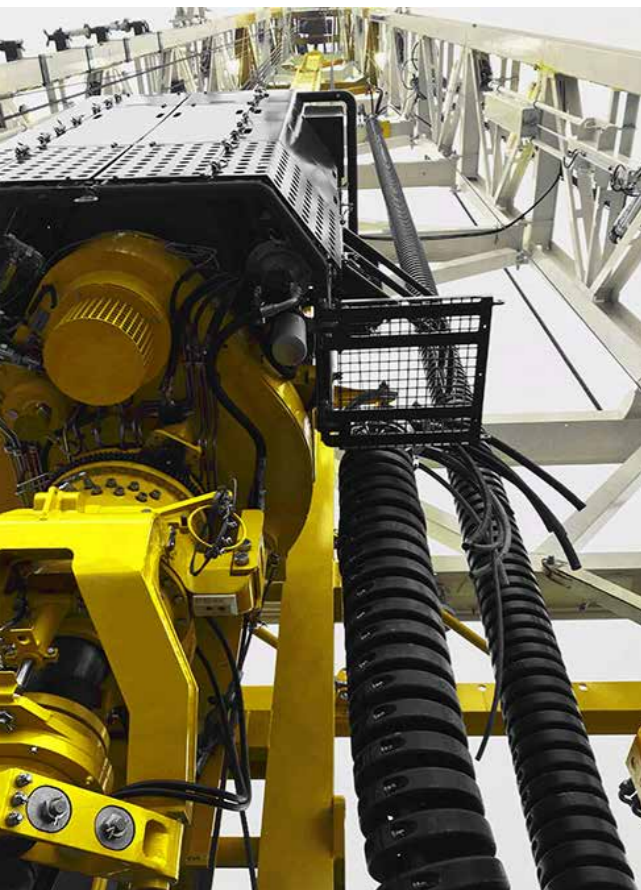
Figure 8: The first e-loop systems are already in operation on land drilling rigs. (Source: igus® GmbH)
