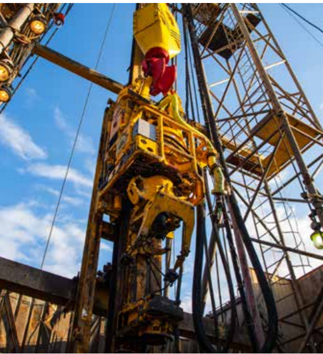
Figure 1: Top drive with service loops and flushing hose on an oil drilling platform (Source: Adobe Stock, Alexandr, 211146059)
