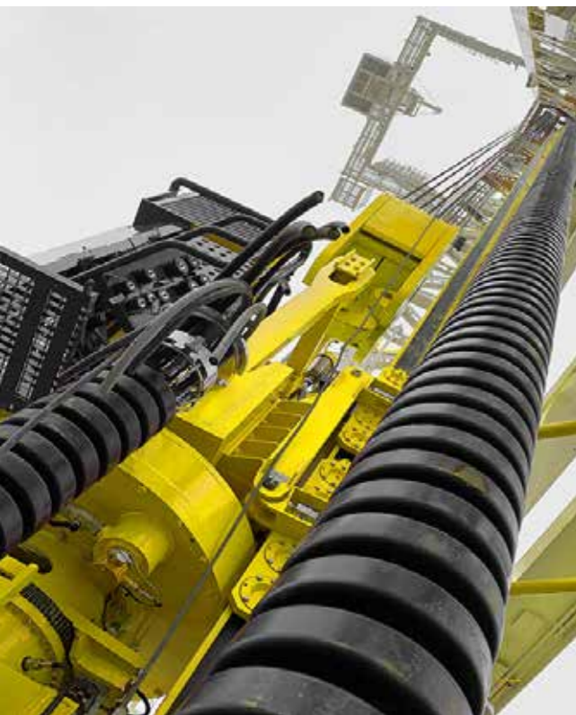
Figure 3: The e-loop system combines all cables into a compact and modular system (Source: igus® GmbH)
