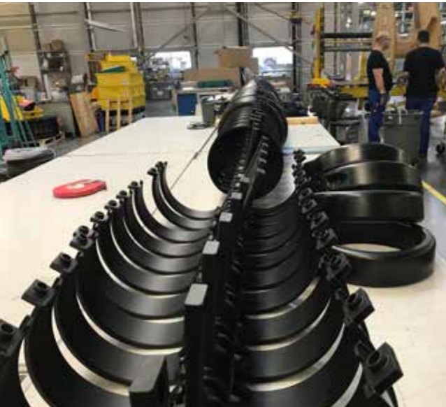
Figure 5: Structure of the e-loop, half-shells with shock-resistant PU attachment (Source: igus® GmbH)
