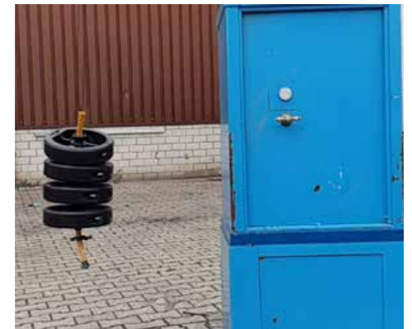
Figure 7: The e-loop survived the breaking test with a strongbox without any problems. (Source: igus® GmbH)
