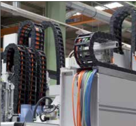
Permanently reliable data transmissions, e.g. with Chainflex® cables harnessed to DriveCliqu standard.
