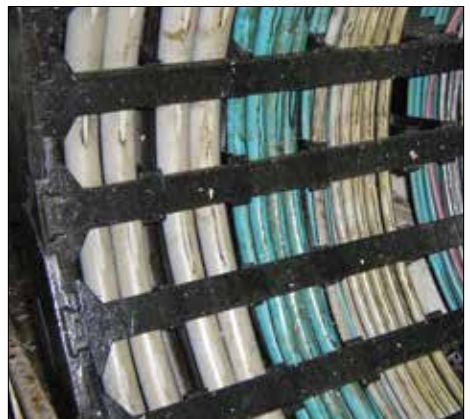
Chainflex® cables are reliable even in oil and coolant.
