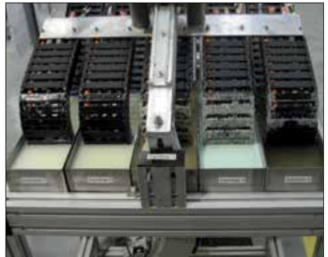
Media resistance testing on Chainflex® cables
