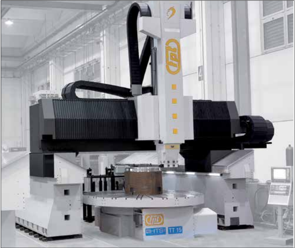
A wide range of E-Chains® in a CNC machine tool – hanging, upright, rotated, and unsupported.
