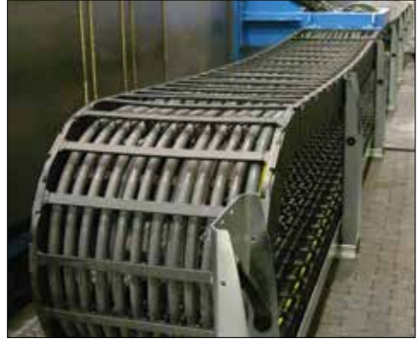
For long travels in the chip area – Guidelok horizontal guides up to 164 ft. (50 m).
