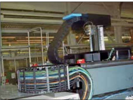
Saving space: the X-axis of the E-Chain® lies on the upper machine cover.
