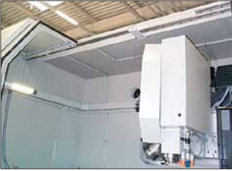
Machine doors with maintenance-free guide using DryLin® linear technology.
