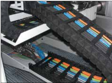
Combined motion with an igus® E6 ReadyChain®.
