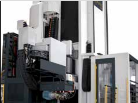
Several E-Chains® and Chainflex® cables in various installation methods.
