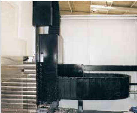
igus® E2 E-Tubes, upright and rotated by 90° in the chip area.
