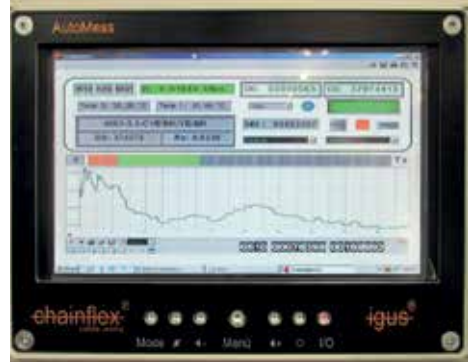
The igus® "AutΩMeS" system tests and records electronic test data in real time.
