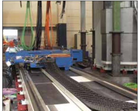
Holding Chainflex® cables in E-Chains® for motion-control applications.
