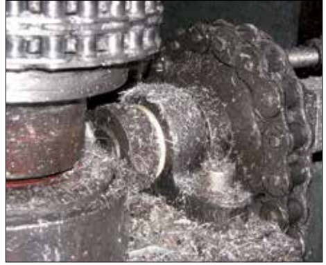
Dry-running igubal® plastic spherical bearings – no chip adhesion.
