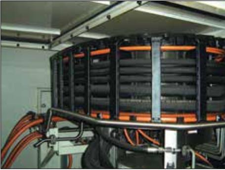
E-Chain® E6 in a CNC grinder: its low weight supports particularly smooth motions.
