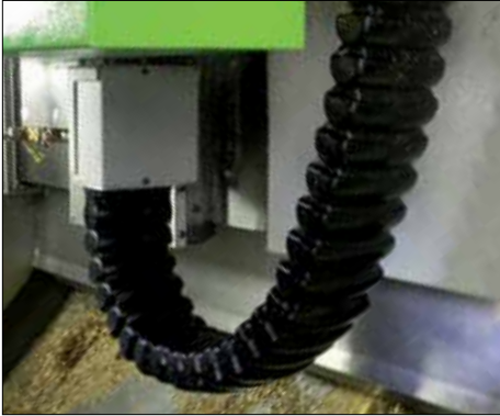
Brass chips and oil/coolant – igus® RX E-Tube protects reliably.
