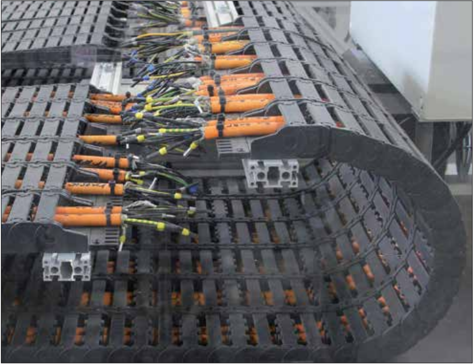
Cable service life test at the igus® lab, Cologne.
