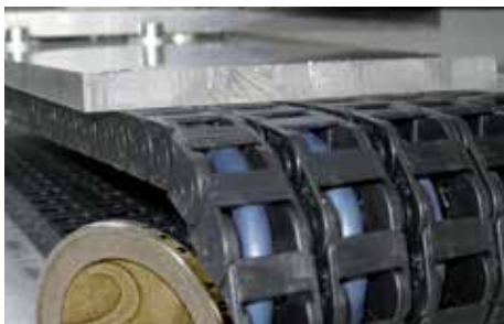
Control cable CF98-05-04 tested in e-chain ® . More than 138 million strokes with a bending factor of 3.2 x d
